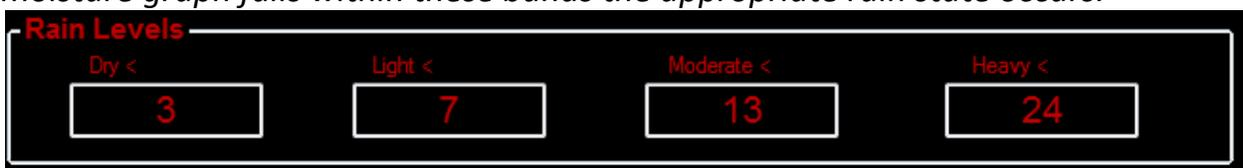
In the above the rain state would be dry as long as the graphed value is less than 3. A value of 8 would be indicated as moderate rain.
