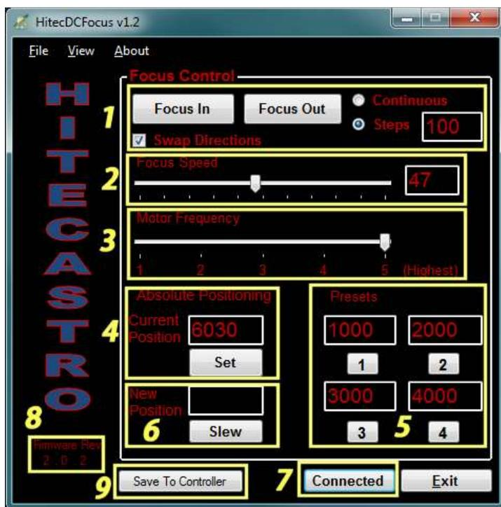
Once you have your power, motor, and USB cable plugged in click the 'Connect' (7) Button. If all is well, the text of the button will change to 'Connected' and the focuser will retrieve the current settings from the unit.
